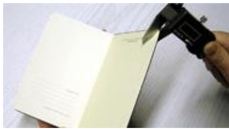
Quality Control. Cover thickness test.
