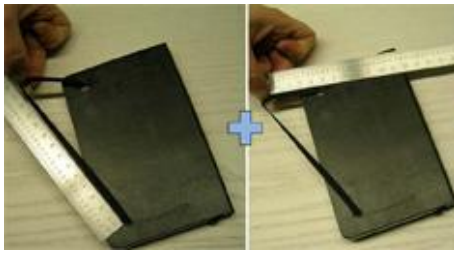
Quality Control. Elastic extension test.
